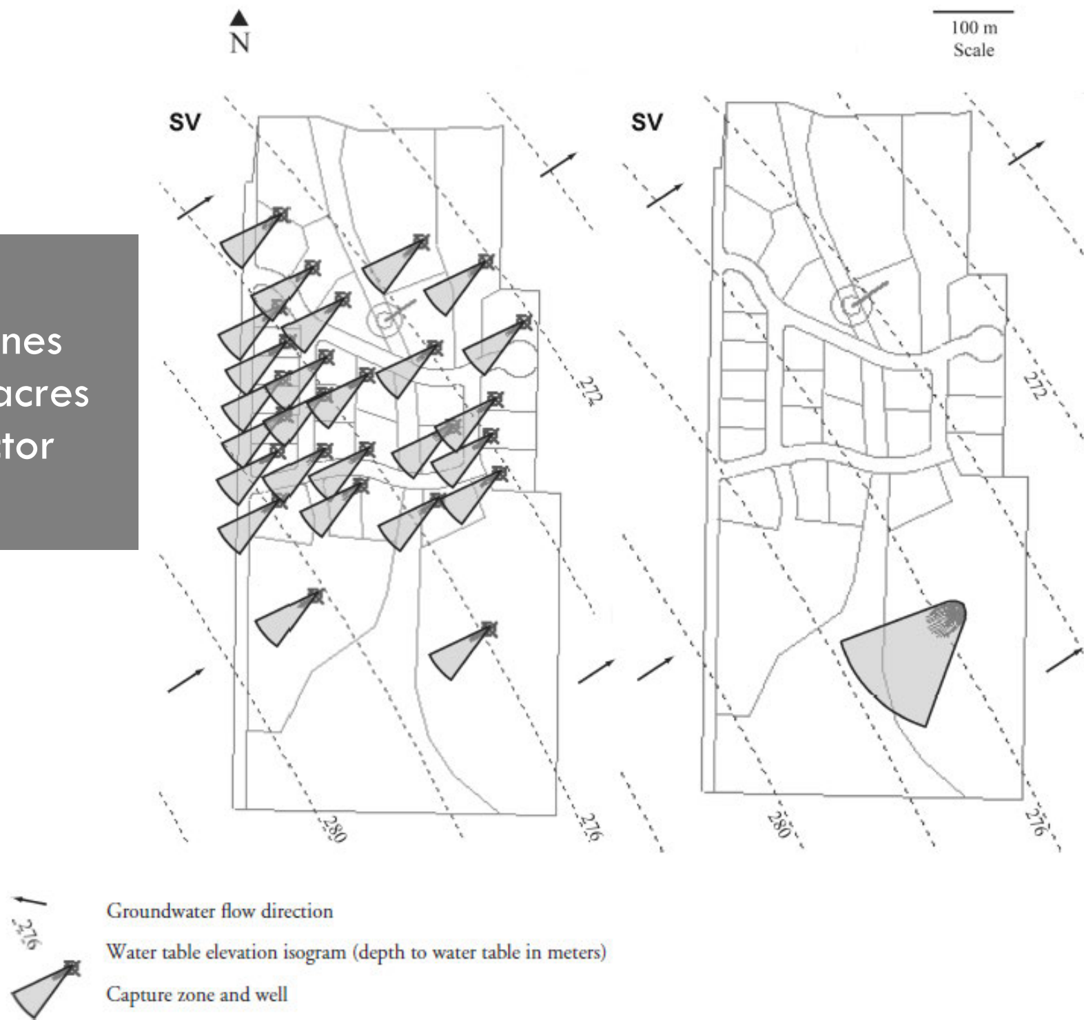
Figure 5. Simulated two-year time-of-travel capture zones for individual wells and community wells.
