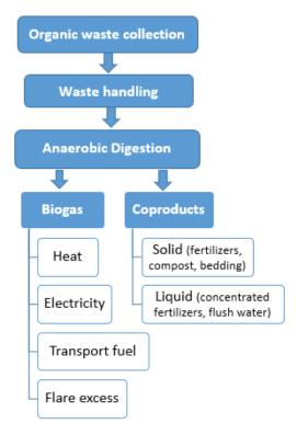
Figure 2: Biogas production steps, process and uses (Adapted from EPA AgStar)<sup>1</sup>
