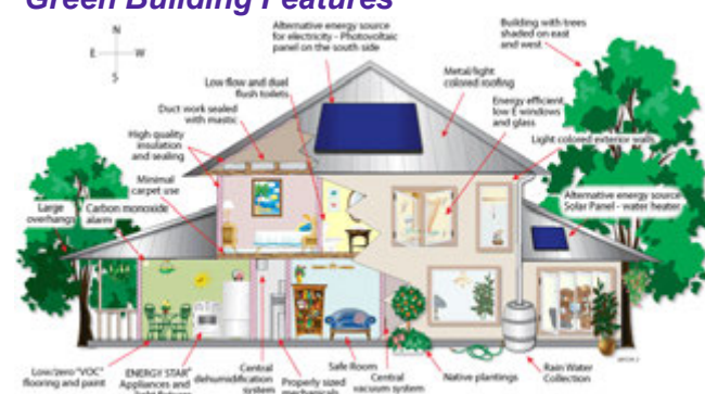
Figure D3 Green Building Features
