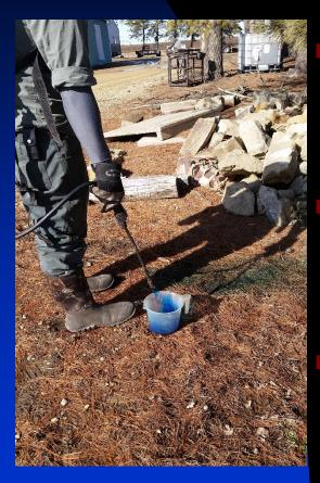
Spray into a measuring pitcher for the length of time it took to spray the 17x20 area
