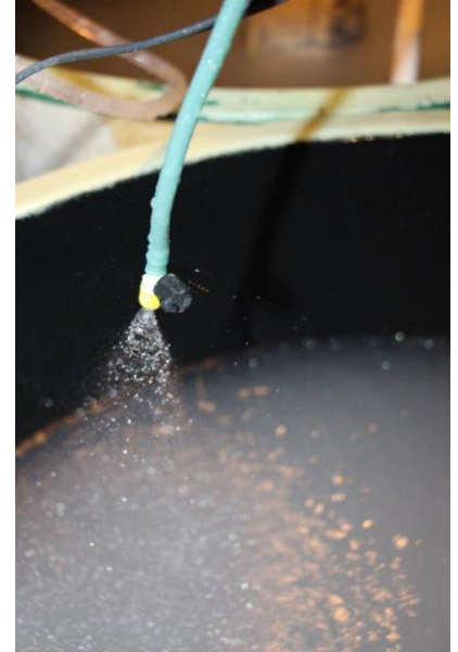
Fig. 26. Spray bar mister directed down at the surface water of the larval tank.
