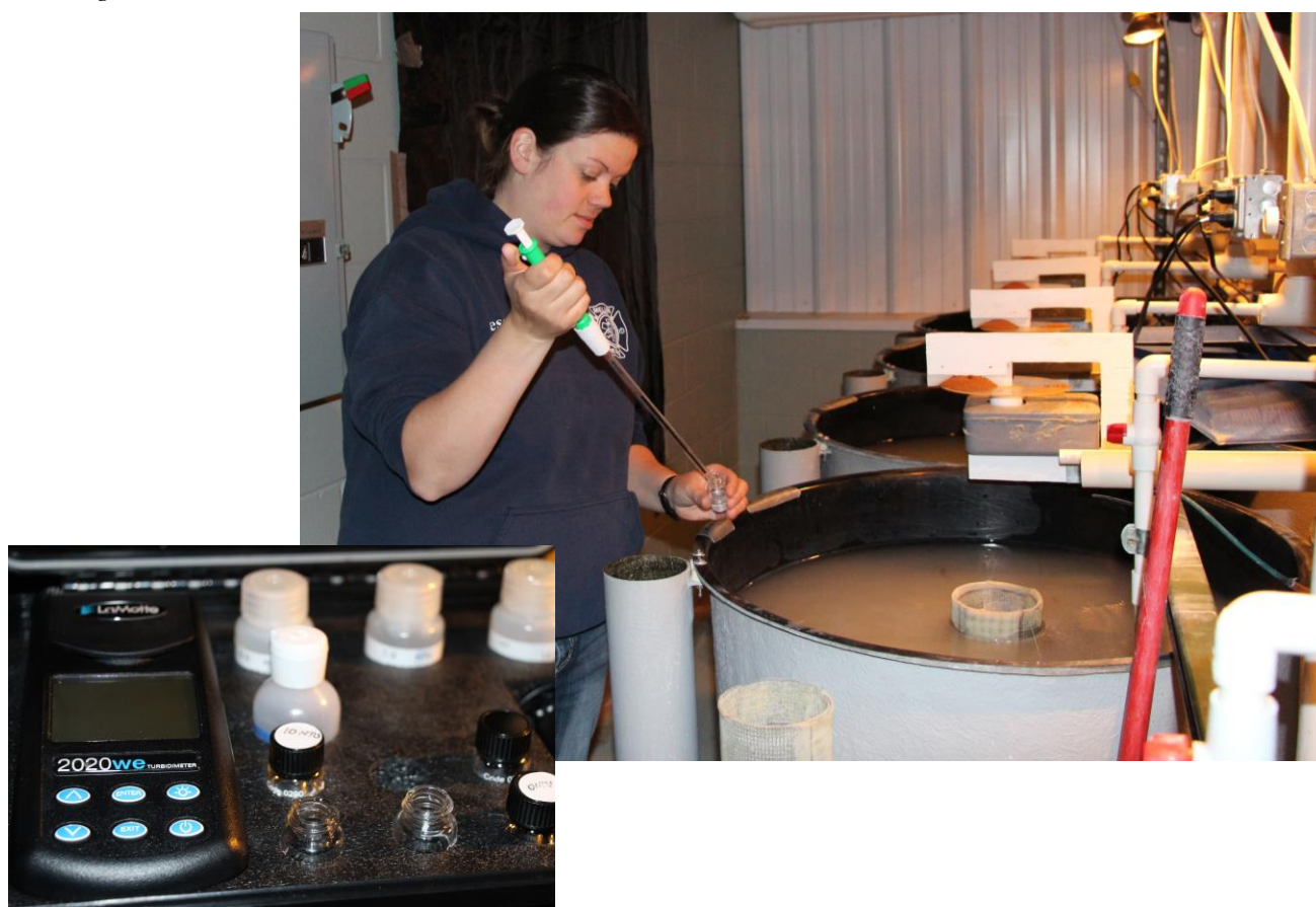
Fig. 40. Turbidity in the larval system is checked daily in a sample of tanks. A pipette is helpful for obtaining a sample from the middle of the water column (top). UWSP NADF uses either Hach or LaMotte brand turbidimeter for checking NTUs (bottom left).
