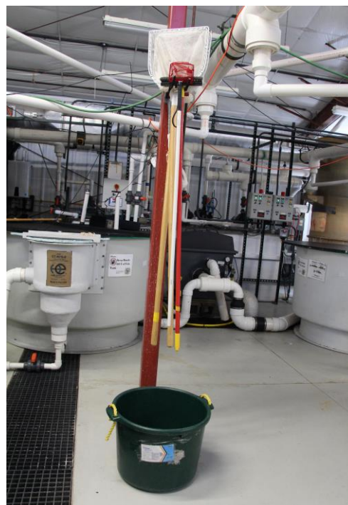
Fig. 63. System equipment is sterilized with an aquaculture approved disinfectant after use and hung up to dry.
