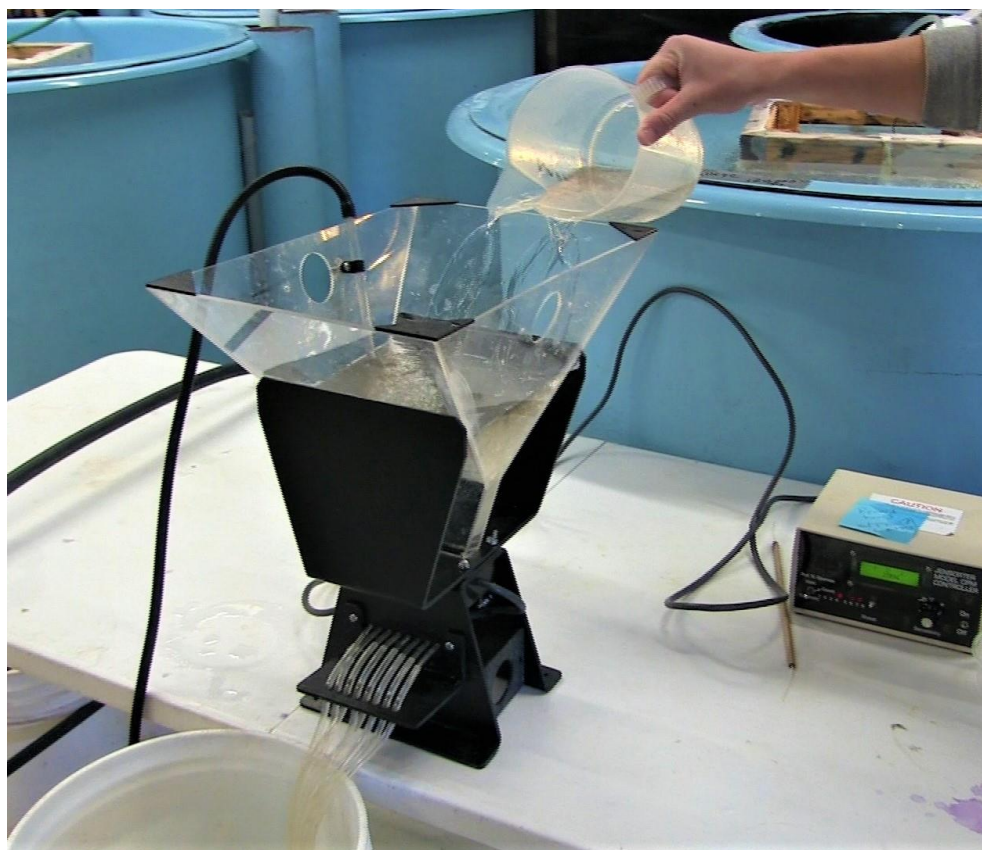
Fig. 19. Once the controller is calibrated, strong swimming fry can be poured into the Jensorter hopper and counted utilizing infra-red detection.
