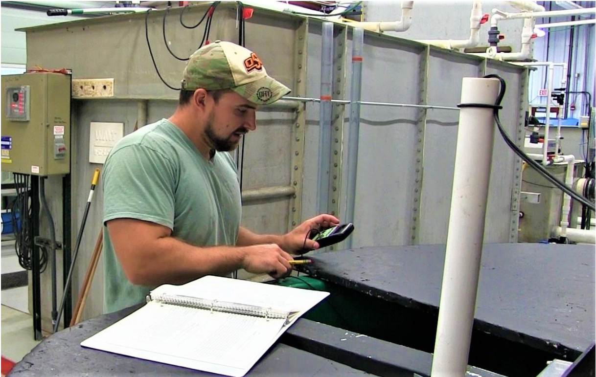
Fig. 5. UWSP NADF Technician, Jared Neibauer, checking pH with PinPoint pH probe in the walleye RAS tanks.
