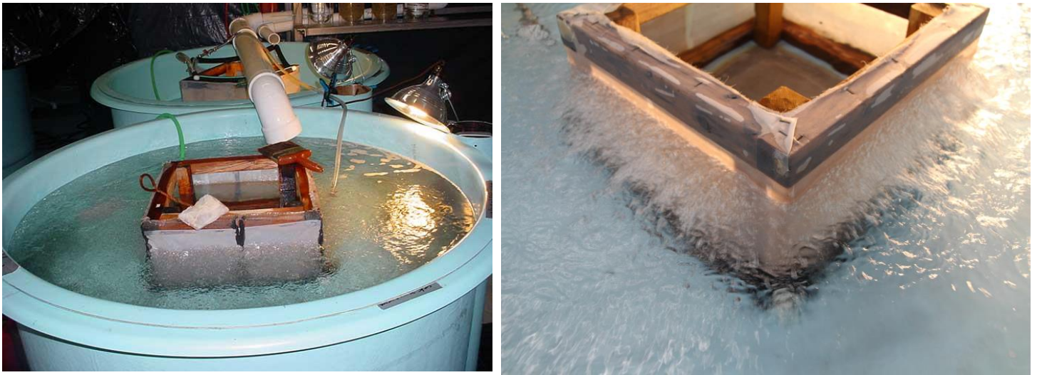
Fig. 17. Photos show bell jar system insert tanks with overhead lighting and a 400micron center box screen. Aeration tubing runs around bottom of the box screen creating a bubble curtain to help keep screen free of debris.
