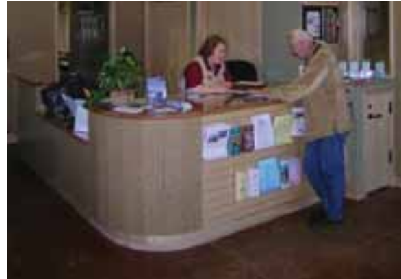
Part of the front desk should be lower to accommodate people in wheelchairs and children, like the left side of this desk at Lebanon Hills Visitor Center in Minnesota. Sales items can be incorporated into the desk.
