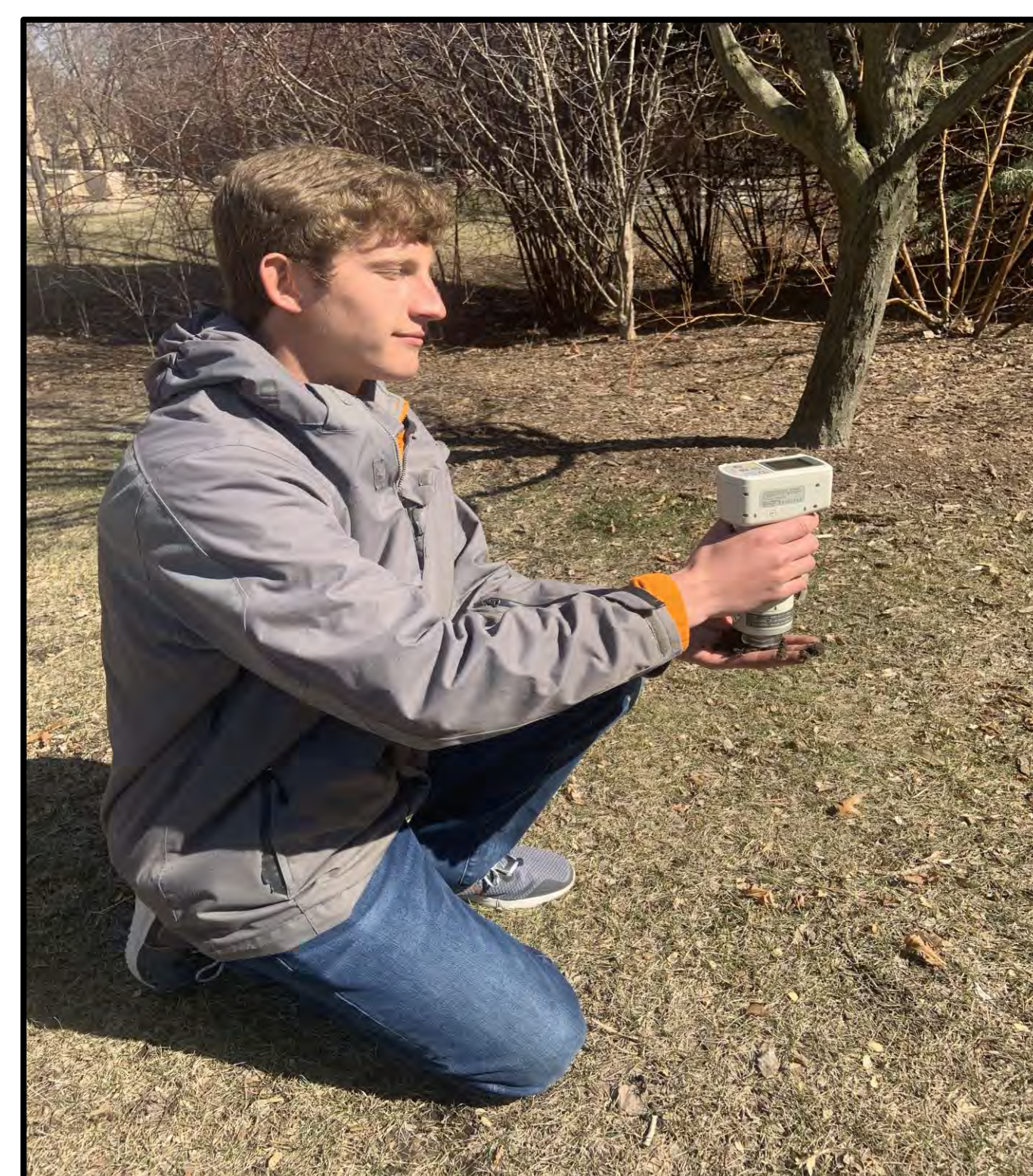
Figure 1. Measuring soil color in the field with the Chroma Meter to predict SOM.
