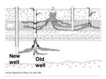
This diagram shows how not properly filling and sealing old wells can contaminate new wells nearby.
