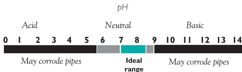
change in acid level. Acidic water is often corrosive (see Corrosivity Index). Iron may also be found at problem levels in acid water. Lab pH values are often slightly higher than would be found at your well.
