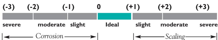
water include pinhole leaks in copper pipes or green stains on plumbing fixtures. Lime precipitate (scale) from hard water is a natural protection against corrosion. Too much scale, however, will partially plug pipes and water heaters, decreasing their efficiency. Water softeners prevent scale buildup, but they can also destroy any protection from corrosion the water may have provided.
