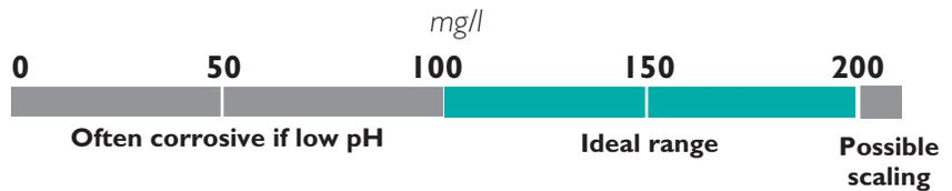
hardness, test for chloride, nitrate and sulfate.
