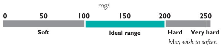
heaters. It also reacts with soap to form a “scum” which decreases soap's cleaning ability, increases bathtub ring and turns white laundry grey. Water that is naturally too soft may be corrosive. The water softening industry measures hardness in grains per gallon. One grain/gallon=17.1 mg/l CaCO<sub>3</sub>.
