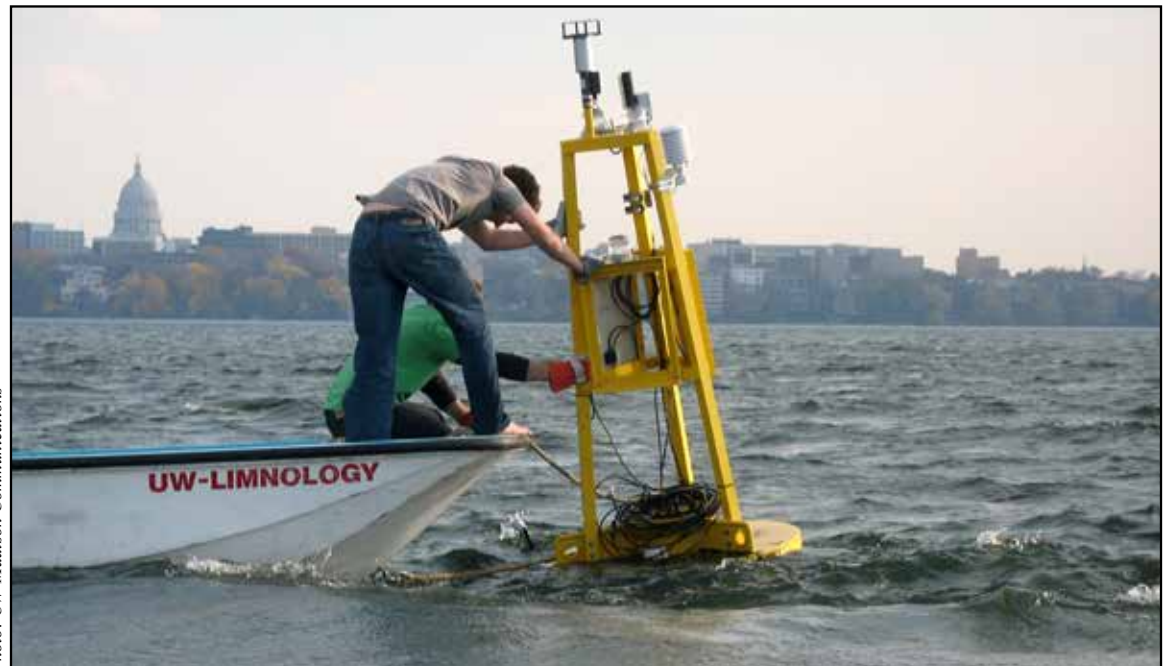
The CFL’s buoy, nicknamed “David Buoy,” keeps track of weather conditions, water temperature, algae growth and chemistry on Lake Mendota throughout the open-water season.
