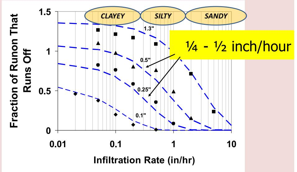
Runon Ratio 500 / 5(w) x 40 (L) The fraction of runon to the secondary buffer that would infiltrate for different storm sizes and infiltration rates (assumes a 500 ft2 impervious area draining to a five foot wide channel, forty feet long and one hour storm of depth shown). Dashed lines show the fitted equation based on soil infiltration rate and storm depth.
