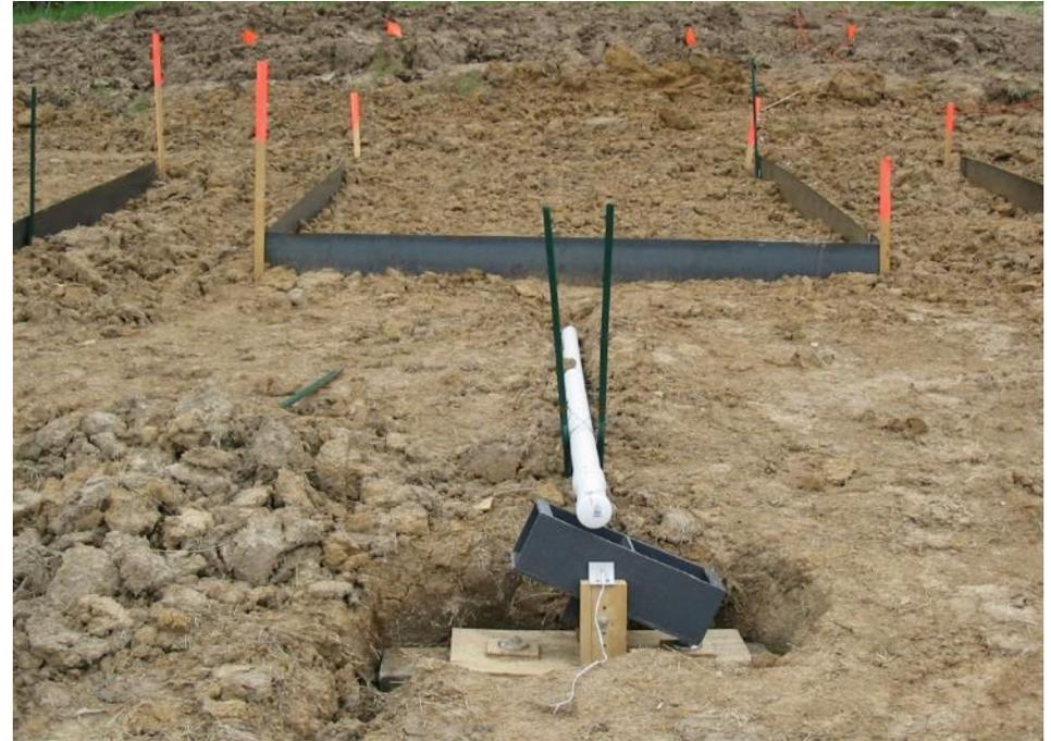
This plot shows the reduction in surface runoff from different approaches to treating compaction.
