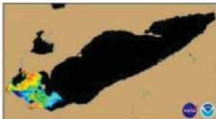
Figure 2. Cyanobacterial Index from NASA MODIS-Terra data collected 24 September, 2017 at 11:55.
