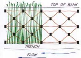
Step 3: Place stake (notched) on 1.0m (3ft.) centers and secure the mattress with twine, rope or wire.
