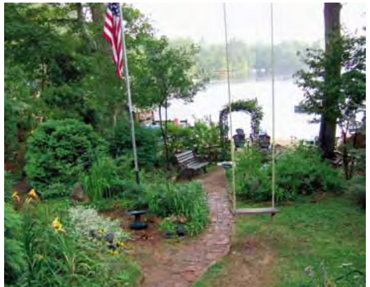
Pathways made of pavers are semi-pervious to water. The path is not straight, so runoff is distributed into vegetated gardens where it infiltrates the ground before reaching the shore.
