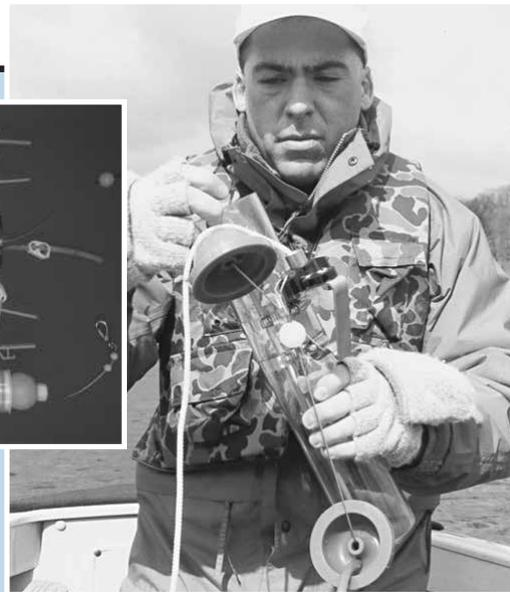
**STEP 2.** Hold the sampler line in one hand and the brass messenger securely in your other hand.
