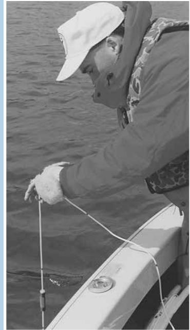
**STEP 5.** Bring the now closed sampler to the surface. Allow time for thermometer to stabilize. Read thermometer. Empty the sampler and repeat steps 1-5 for each depth.
