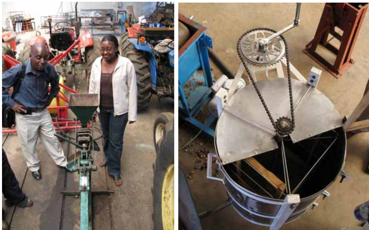
Figure 4: Former GEM-sponsored, JKUAT intern, Judith Mwendu, and Philip Ndichu inspect a manual oil seed press and bicycle-gear honey extractor, both appropriate-scale technologies that could be of great use at Nyumbani Village.
