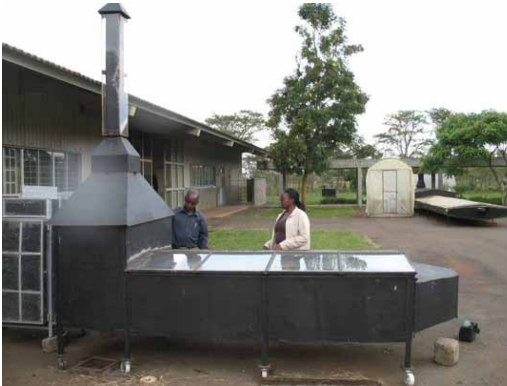
Figure 3: Large-scale solar dehydrator built by students at Jomo Kenyatta University of Agriculture and Technology.
