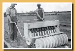
Mechanical seed drills planted multiple rows of seeds to the correct depth (1931 photo).
