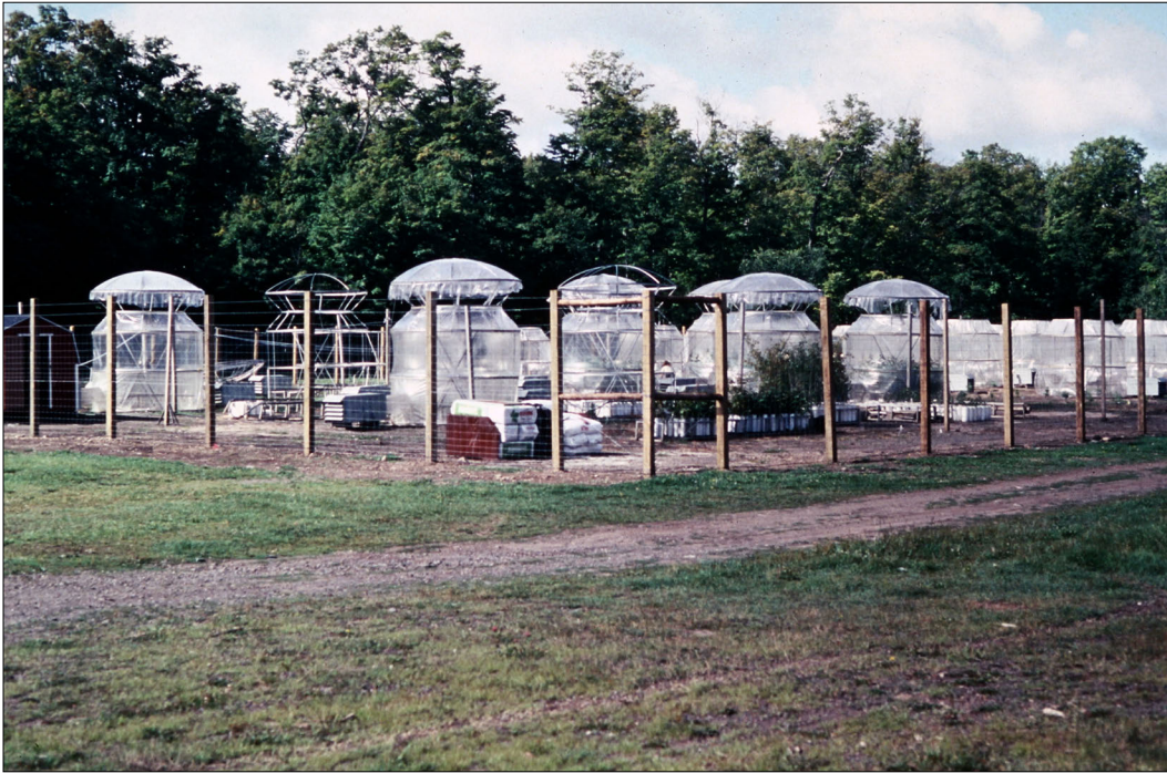
Figure 60. —Open-top chambers for studying elevated levels of ozone and carbon dioxide in 1993, part of the Physiological Mechanisms of Growth and Multiple Stress Responses project at the lab. Courtesy photograph by J.G. Isebrands.
