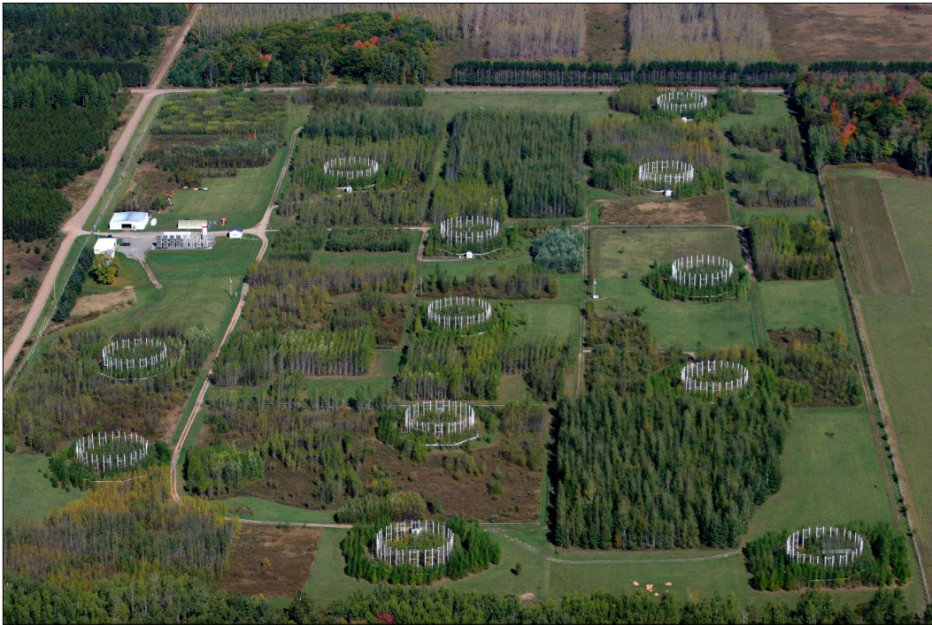
Figure 61. —The Aspen Free-Air Carbon Dioxide and Ozone Enrichment (Aspen FACE) experiment site, consisting of 12 circular plots planted with aspen, birch, and maple trees surrounded by PVC pipes that vented carbon dioxide and ozone gas. Courtesy photograph by John Couture, UW-Madison.
