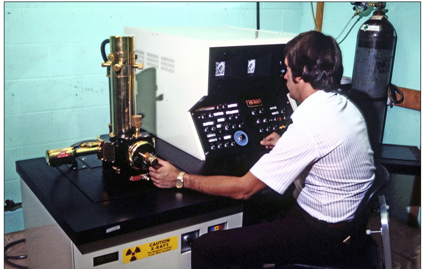
Figure 75. —Ronald “Ron” Teclaw, research biologist, using a scanning electron microscope as part of the Physiology and Raw Material Evaluation of Intensively Cultured Plantations project in 1980. At the time, the Rhinelander field laboratory had one of only twenty scanning electron microscopes in Wisconsin. Courtesy photograph by J.G. Isebrands.
