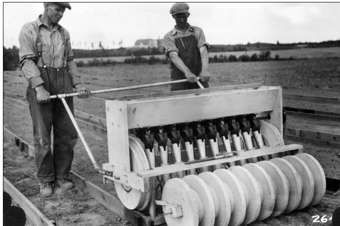
Figure 10. —Nursery staff using a 10-row mechanical seed drill to plant the seed beds, 1932. USDA Forest Service photo archives.
