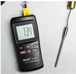
When lowering the probe into the water, please manually feed out loops of cable from the spool, instead of spinning the spool itself. Spinning it will cause the cable to twist between the spool and the display unit.
