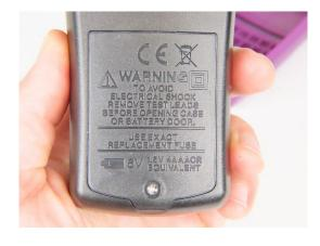
There is a small Phillips-head screw in the back battery cover. Remove the screw and lift the bottom of the battery cover to access the batteries. The unit takes 4 AAA batteries.
