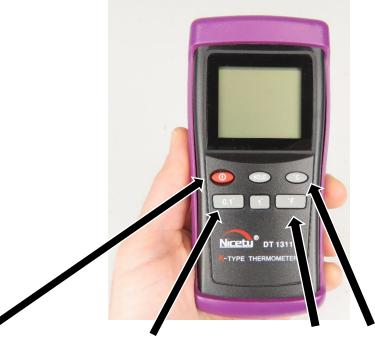
Power button – Turns the unit on or off. **0.1-degree button** – Changes format to display temperature in tenths of a degree.
