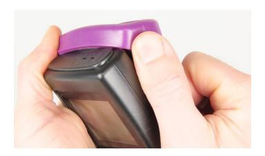
Hold the unit in your hand and press back on the top corners. The unit will separate from the protective case. To put the unit back into the case, just slide the top end in and then the bottom end.
