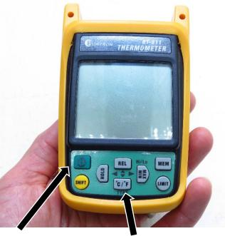
Power button – Turns the unit on or off. Celsius – Fahrenheit button – Push this to change the display to Celsius or Fahrenheit degrees
