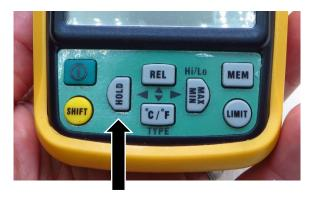
If you accidentally press the HOLD button, it will not display the current temperature. Push the HOLD button again to reset it.
