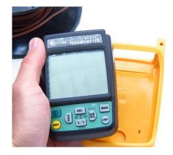
To put the unit back into the case, just press one end in and then the other.
