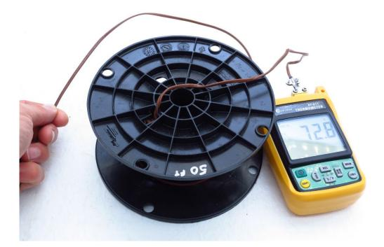
When lowering the probe into the water, please manually feed out loops of cable from the spool, instead of spinning the spool itself. Spinning it will cause the cable to twist between the spool and the display unit.
